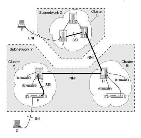
Figure 3-4. Using Static Route Mappings to Connect User Devices
